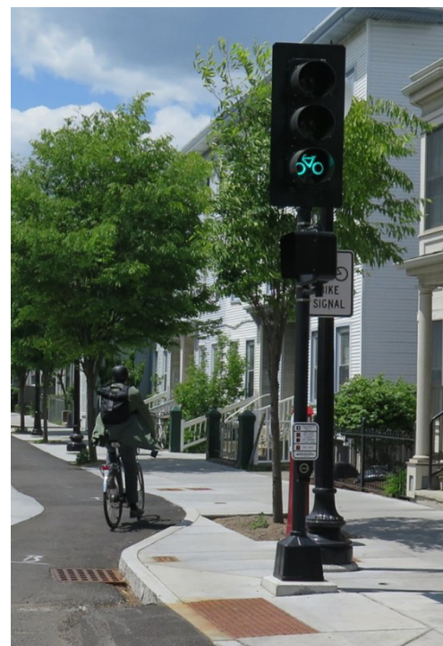
Western Avenue separated bicycle lane in Cambridge. From this vantage point, the bicycle lane transitions from road grade at the intersection to sidewalk grade. Street trees and furniture provide a physical barrier between the bicycle lane and the adjacent sidewalk, and the asphalt and concrete materials provide a visual barrier as well.
