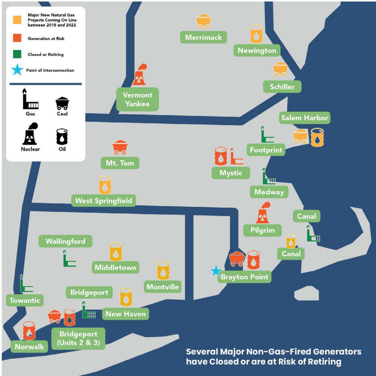
**Figure 3-1. Generators at Risk of Retiring or Already Retired, per ISO-NE<sup>1</sup>**
