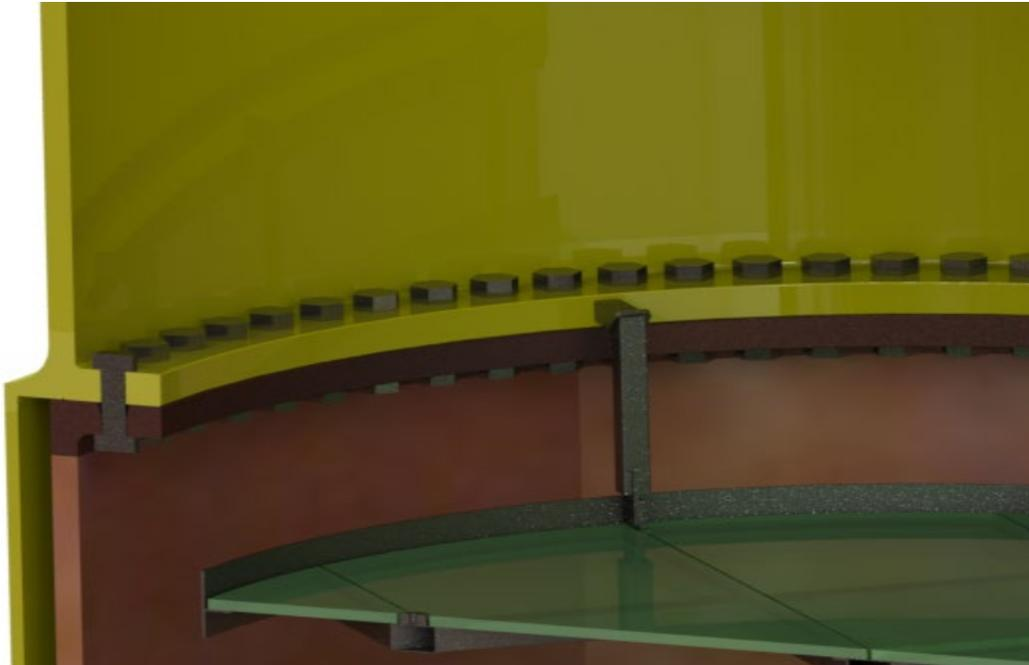
**Figure 10-12. Bolted Connection Between the Transition Piece and Monopile Flange**
