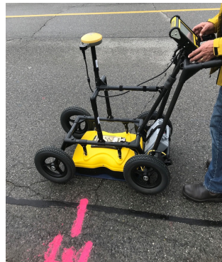
Push-Cart Ground Penetrating Radar Systems are designed to detect the location of buried facilities and structures.
