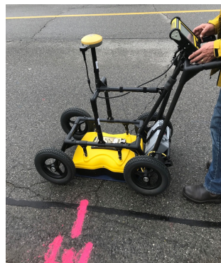
Push-Cart Ground Penetrating Radar Systems are designed to detect the location of buried facilities and structures.
