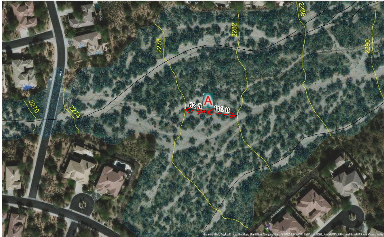
Figure 11: Measuring a Subject between BFEs in overbank areas when the floodplain is derived from 2-D models.
