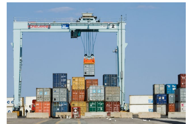
Hybrid RTG Retrofits
