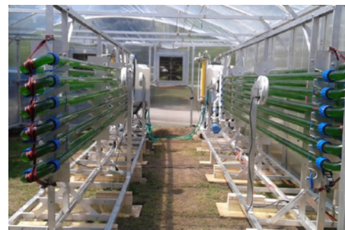
Photobioreactor consisting of the control reactor with bottled CO2 on the left and flue gas CO2 on the right
