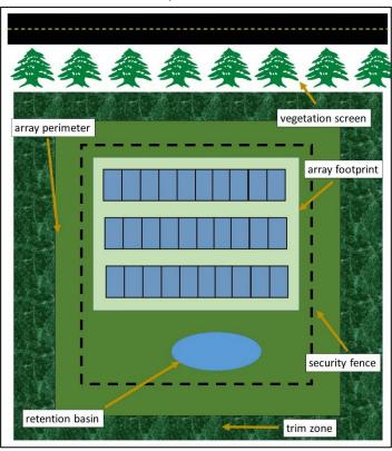
Array footprint – The area beneath the solar PV panels, between adjacent rows of panels, and immediately surrounding the array is typically reduced to bare ground during facility construction. This area can be planted with low-growing (under 36" high) wildflowers and bunchgrasses to prevent shading of panels.
